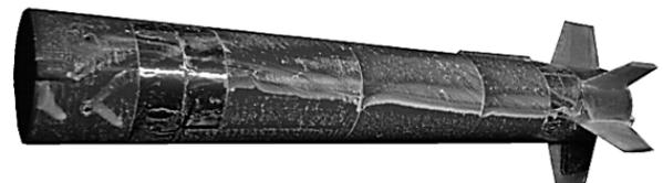
Figura 10 - ensayo de oil flow ( $\alpha=45^\circ$ ).
