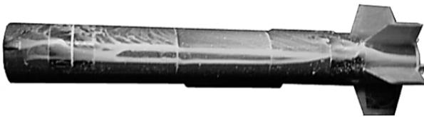
Figura 11 - ensayo de oil flow ( $\alpha=90^\circ$ )
