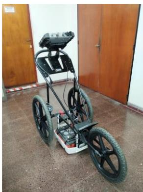
Figura 2– Antena digital HS 350
